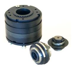
Safegard series of overload clutches are designed to be fully interchangeable with other European manufacturers. Using a number of balls on unsynchronized units, and random positioned rollers on synchronized units, enables high torques and operating speeds to be achieved with compact units. Units with 10 different operating modes, have different flange connections, or Flexible Shaft Couplings, with finish bore and keyway; or clamping bush for shafts from 10 to 200mm.
