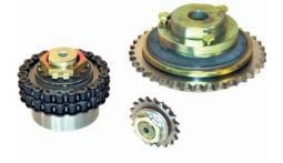
The Morse Torque Limiter is a protection device that limits torque transmitted in a drive, by slipping when the torque exceeds a preset value, due to shock loads, overloads, or machine jams. It automatically re-engages when the overload has passed. Torque Limiters prevent machine damage and costly breakdown time.
