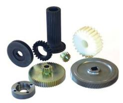
Straight cut bevel and mitre gears manufactured to the Gleason system in medium carbon steel enable simple right angle transfer of drives, with drive ratios from 1:1 up to 4:1 reduction.
